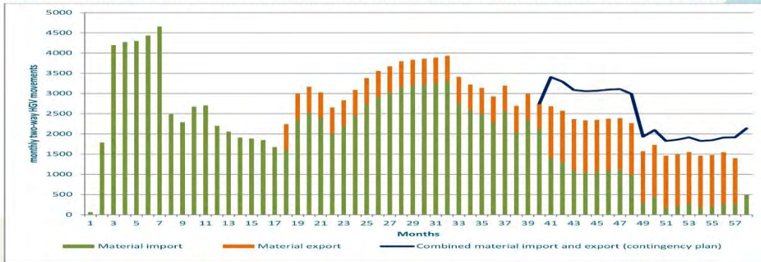
Chart 1 Monthly HGV flows, Mine and Intermediate MTS Shaft Sites, combined material delivery and export
